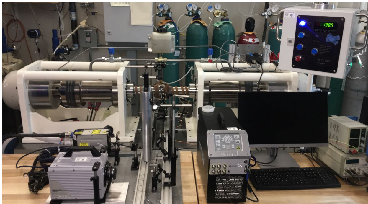
Figure 1. Photograph of the rapid compression machine experimental setup.
