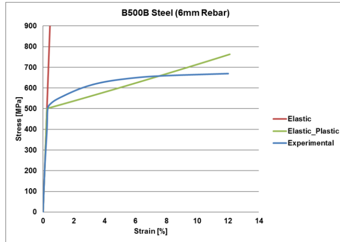
Figure 4-41: B500B Steel Elastic-Plastic Model for 6mm Rebar.
