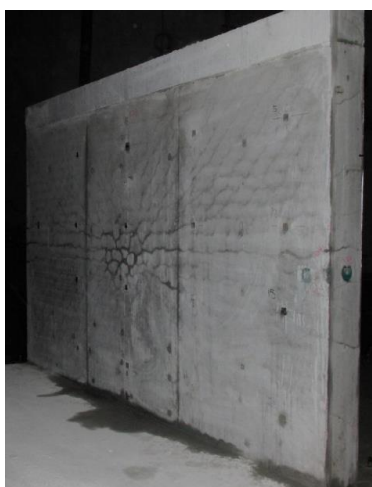
Figure 4-60: Experimental damage on the back face of the impact wall from the 170 m/s missile impact
