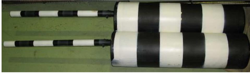
Figure 2-12: IRSN VTT Punching Test Missiles.
