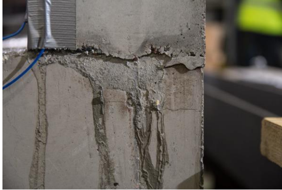
Figure 4-173: Bottom of the front face where it meets the bottom of the mockup showing a complete crack through the concrete.
