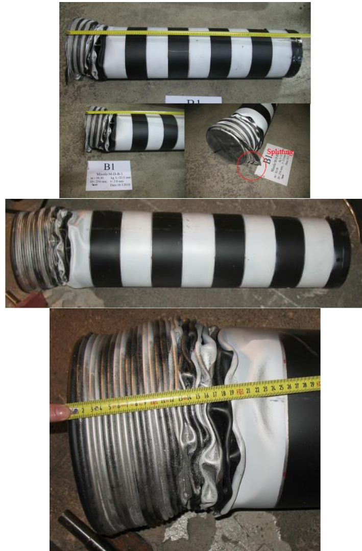
Figure 3-35: Deformed/Post-Impact VTT Flexural Mode Impact Missiles (Top: Test B1; Bottom: Test B2).
