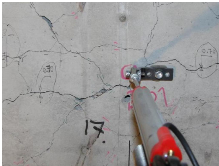
Figure 4-172: Close-up view of the cracking pattern on the back of the impact face. The instrument in the image is a displacement transducer.
