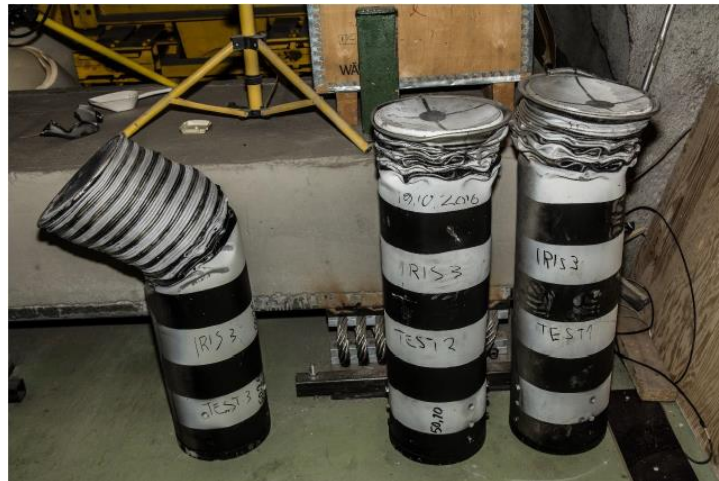
Figure 4-80: Experimental crushed missiles. Left to right: 170 m/s, 90 m/s, 90 m/s.
