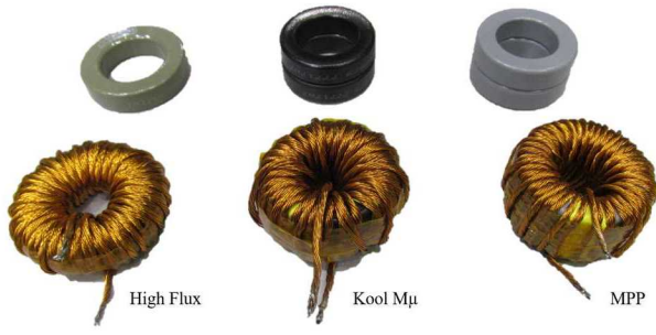
Fig.8 5 kW boost inductor design comparison between P1 (Kool Mμ), P2 (MPP), and P3 (High Flux) prototypes.
