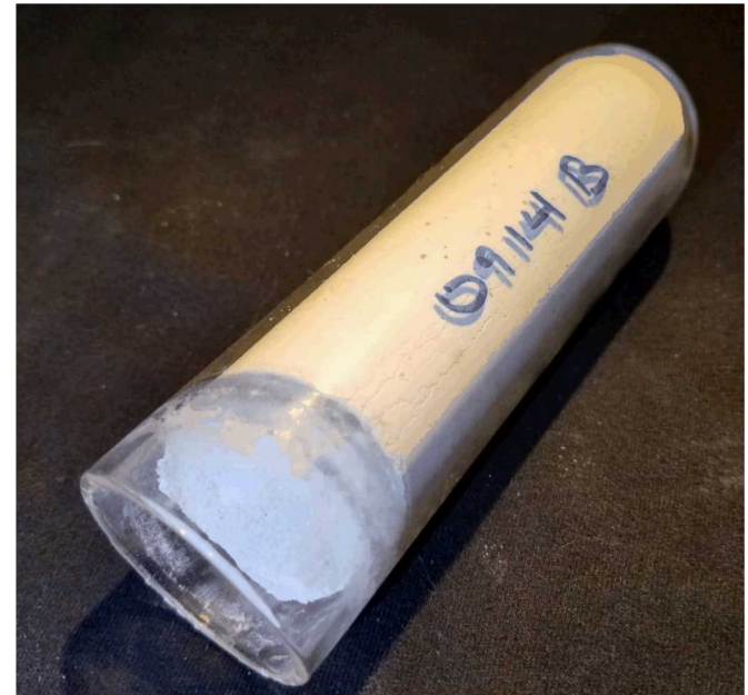
APC sample in Pyrex tube (1.25 in x 5 in) after setting and curing.
