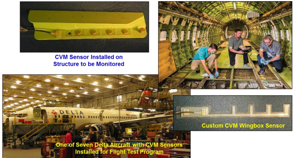
Figure 2-23. Sample Aircraft Application Deploying CVM System to Monitor Cracks on Wing Box Fittings
