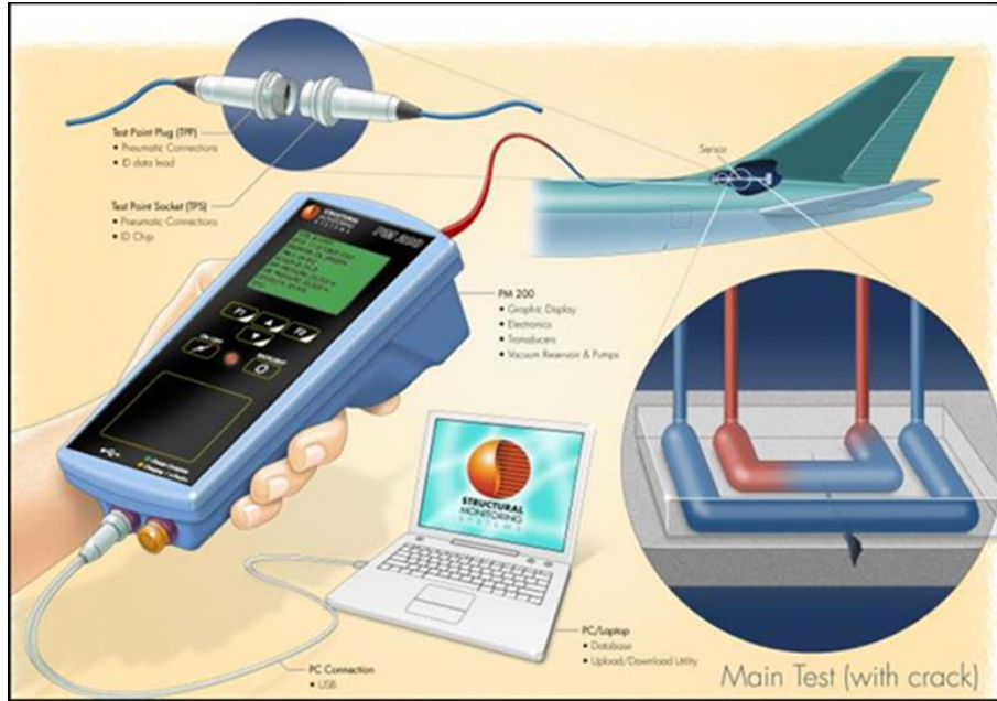
Figure 2-12. Comparative Vacuum Monitoring System
