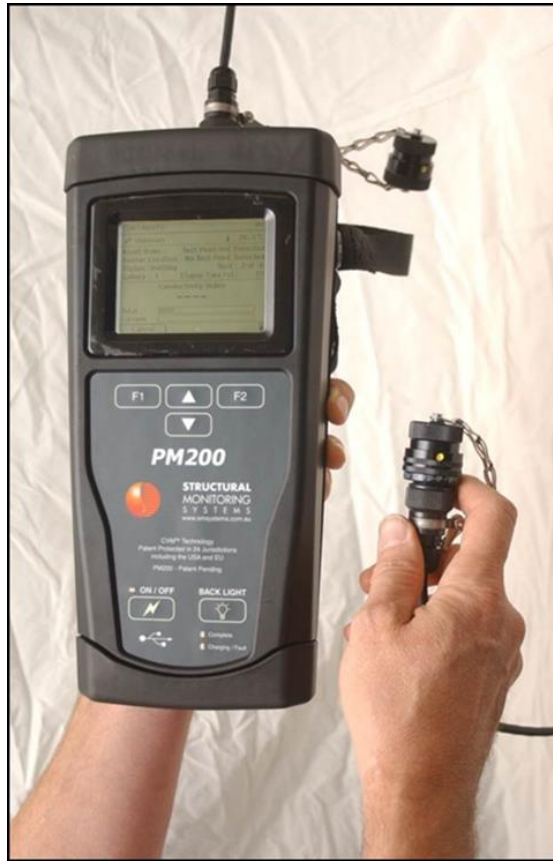
Figure 2-15. PM200 Device Used to Interrogate CVM Sensors and Perform Structural Monitoring
