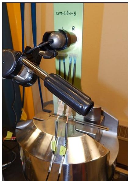
Figure 4-14. Set-Up of Microscope Camera Used to Aid Crack Length Measurements
