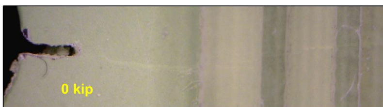
Cracks viewed under load to track growth and show engagement with CVM galleries
