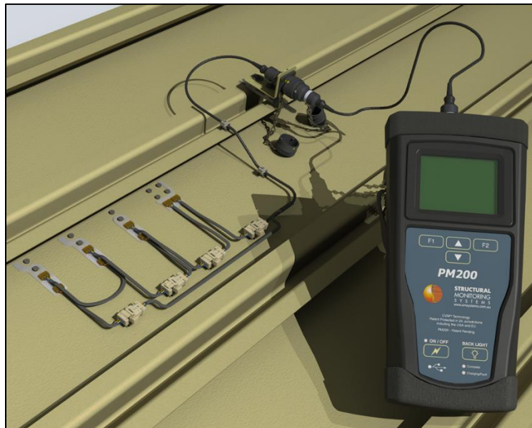
Figure 2-13. On-Board CVM Sensor Network with Aircraft-on-Ground Connection to PM-200 Monitoring Device Using SLS Connectors
