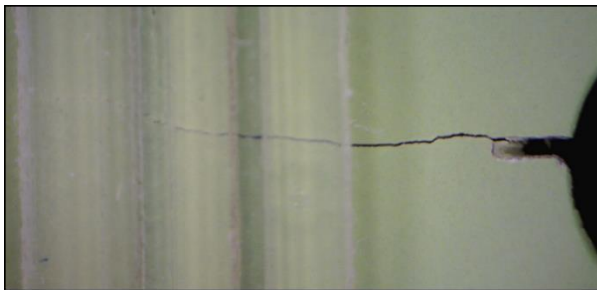
Figure 4-16. Sample Crack Growth and CVM Response Data Recorded for Each Test Specimen – Straight Nut Plate Example 1
