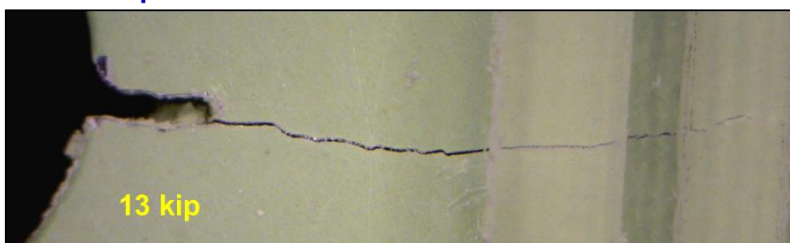
Microscope Camera Records Crack Growth
