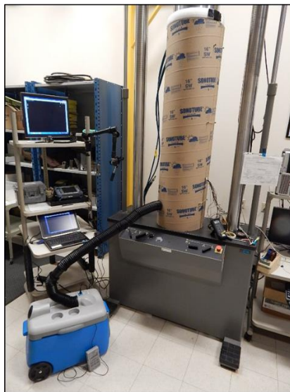
Figure 6-74. Equipment Set-Up Used to Produce Hot and Cold Temperature Extremes
