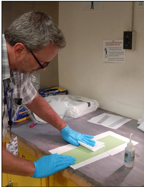
Figure 4-6. Cleaning After Light Primer Sanding for CVM Installation
