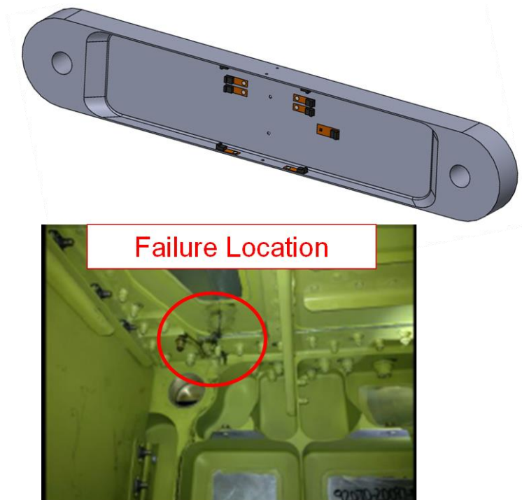
Figure 3-15. Global PZT Crack Monitoring Application on Rotorcraft Beam
