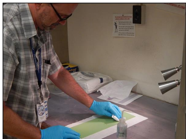
Step 2: To remove any grease, dirt, or any contaminants prior to sanding, wipe in one direction to remove solvent and dirt.
