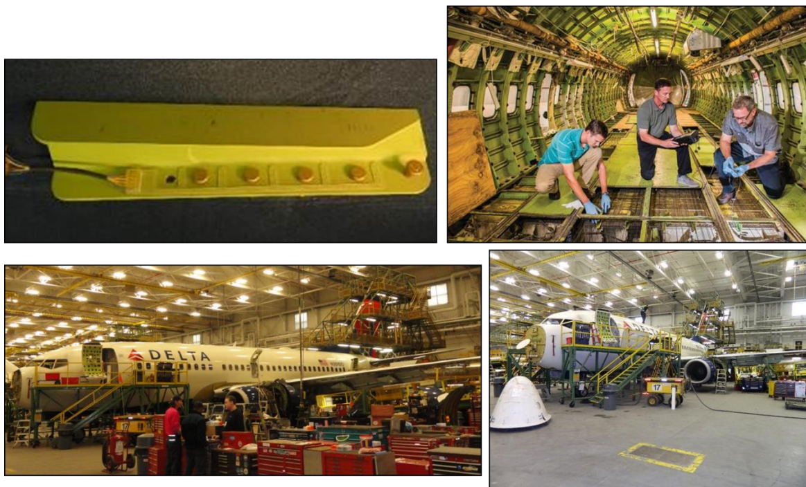
Figure 5-25. Overview of CVM Sensor Installations on Wing Box Fittings at Delta Facility
