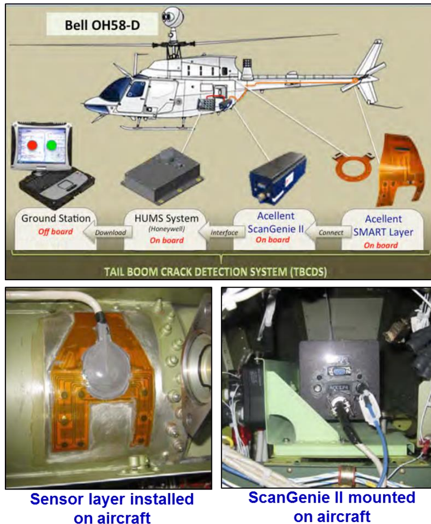
Figure 2-42. PZT Application on OH-58 Tailboom
