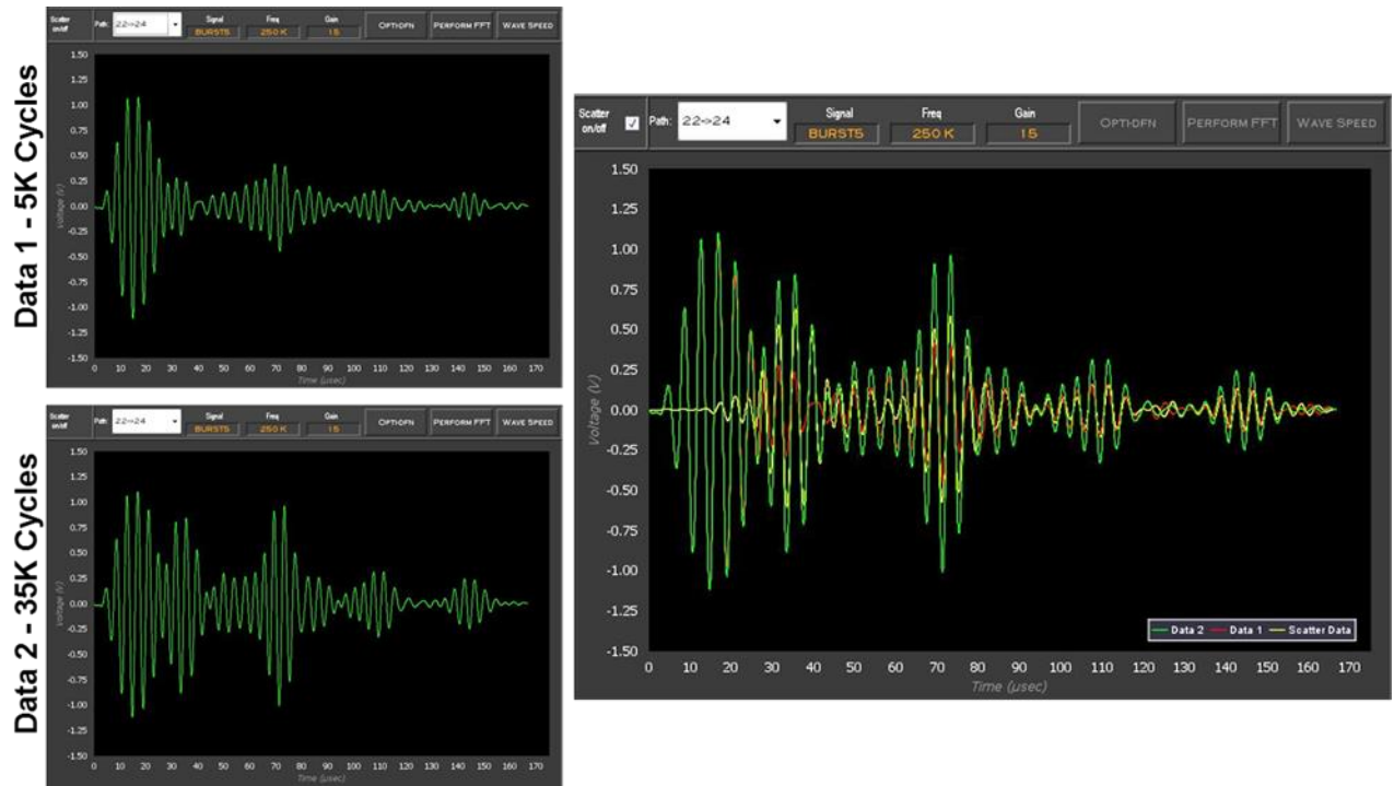
Figure 2-35. Change in PZT Signals from their Baseline (Undamaged) Signatures are Used to Determine a Damage Index - Change in PZT Signal is Represented by Yellow Waveform
