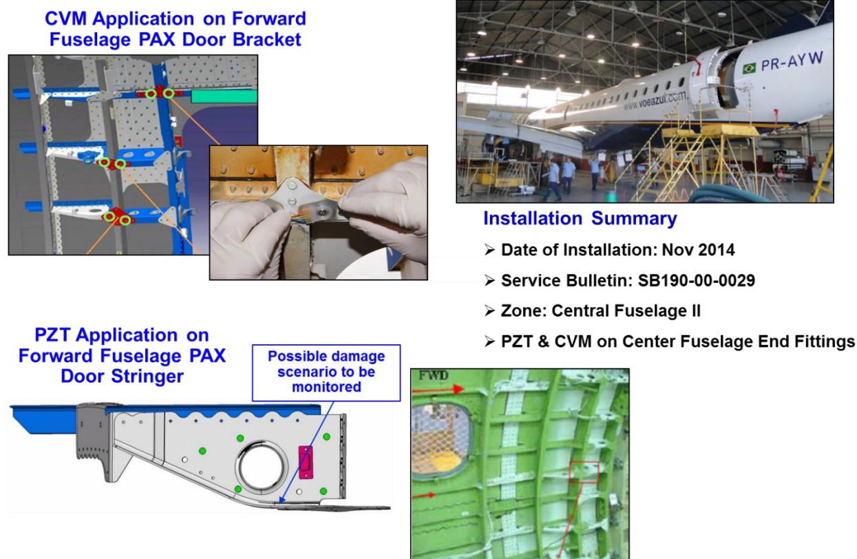
Figure 2-41. Embraer Damage Detection Applications – CVM & PZT Flight Tests – Azul Aircraft PR-AYW
