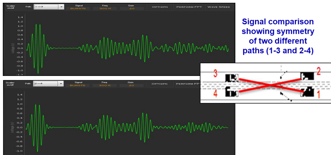
Figure 6-4. Check of PZT Signal Quality – Pitch-Catch Mode on Rotorcraft Beam Top Flange
