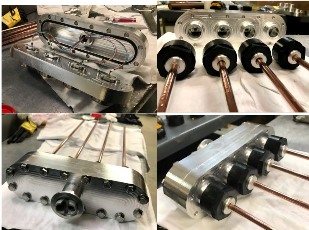
Figure 56 Modular diagnostic head assembly with B-dot probes
