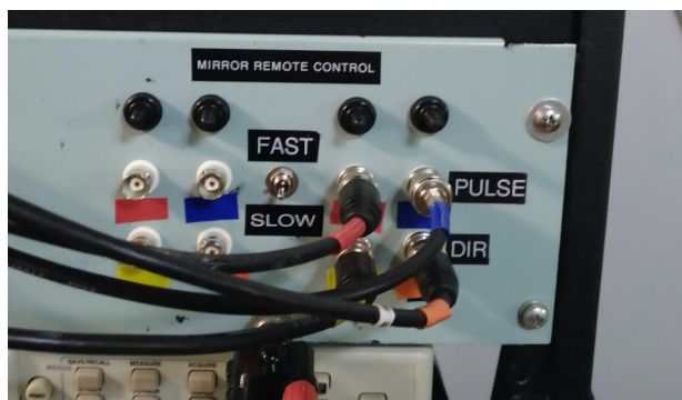
Figure 50 Screen room control system developed for motorized mirror mounts.
