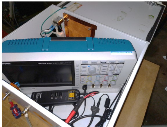
Figure 69 Tektronix TBS2000B differential probe and shielded box.
