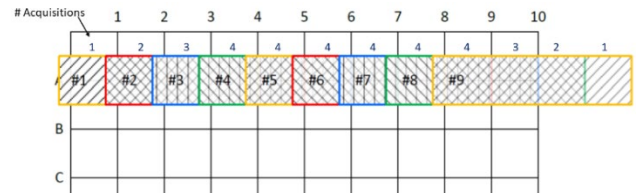
Fig. 5. Illustration of how MIRA is moved horizontally along a gridline, resulting in collection of multiple acquisitions for certain regions.
