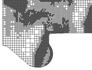
Figure 3.8: Representative GM 1.9L Converge simulation sector mesh at 50 deg. ATDC
