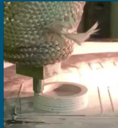
ceramic-thermoplastic 3D (CT3D) printing alumina
