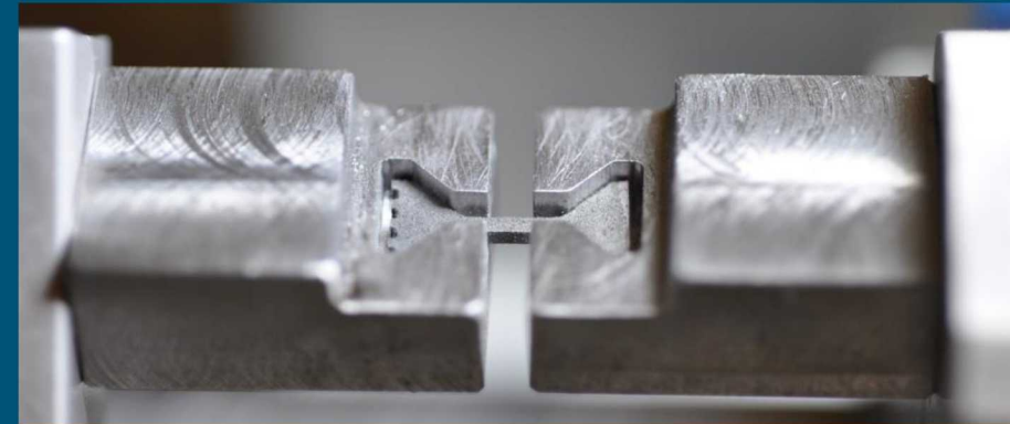
grippers w/ 1x1 mm gage section sample for testing
