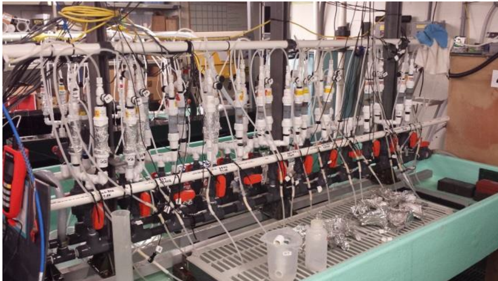
Figure 7. Flow-through column exposure system.
