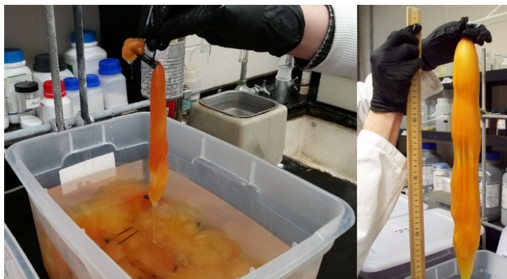
Figure 4. Left panel — 4–6 g masses of adsorbent synthesized using a 2 L reaction vessel. Right Panel — 50 cm long, 40–80 g braids synthesized using a 20 L reactor.
