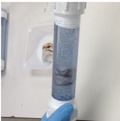
Figure 8. Nominal one-inch ID (2.28 cm actual diameter) flow-through columns packed with fiber adsorbent material.
