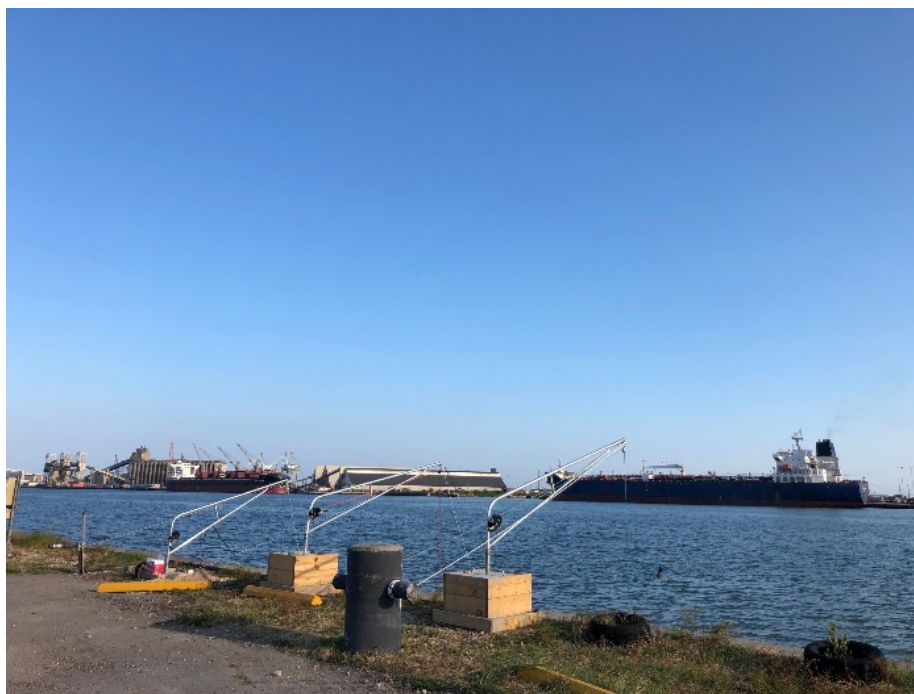
Figure 25. Three customized davits were installed on the pier near the deployment site.
