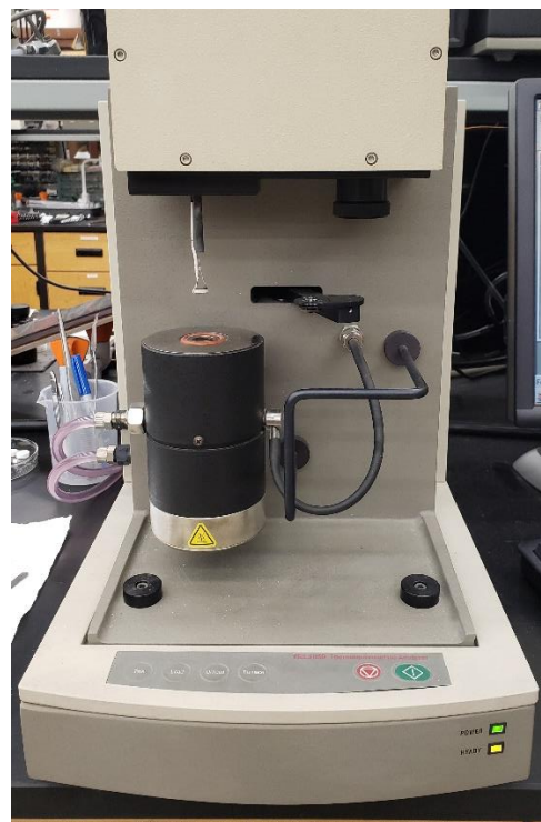
Figure 17. Thermogravimetric analyzer measures mass of material in a small hanging pan while heating. Each fuel was pipetted onto a pan and the chamber held at 60^\circ\text{C} until fully evaporated.
