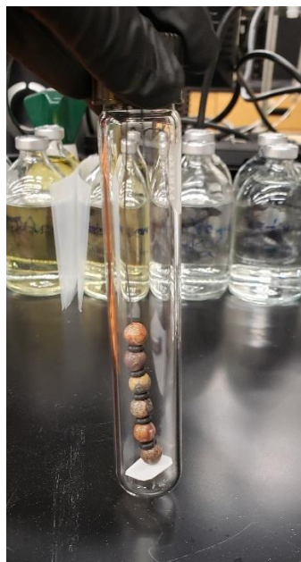
Figure 19. Interactions between o-ring samples, in a single fuel, were reduced by spacing the samples in each test tube with agate beads.
