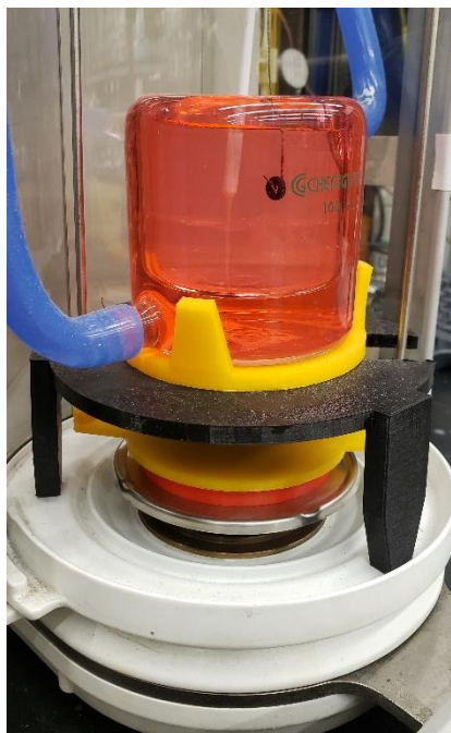
Figure 21. The density of each o-ring is measured while submerged in distilled water.
