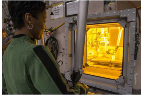
Figure 2: Real-world image of remote manipulator arm. Image credit: Savannah River National Laboratory via Twitter: https://twitter.com/srnlab/status/983767392265306112
