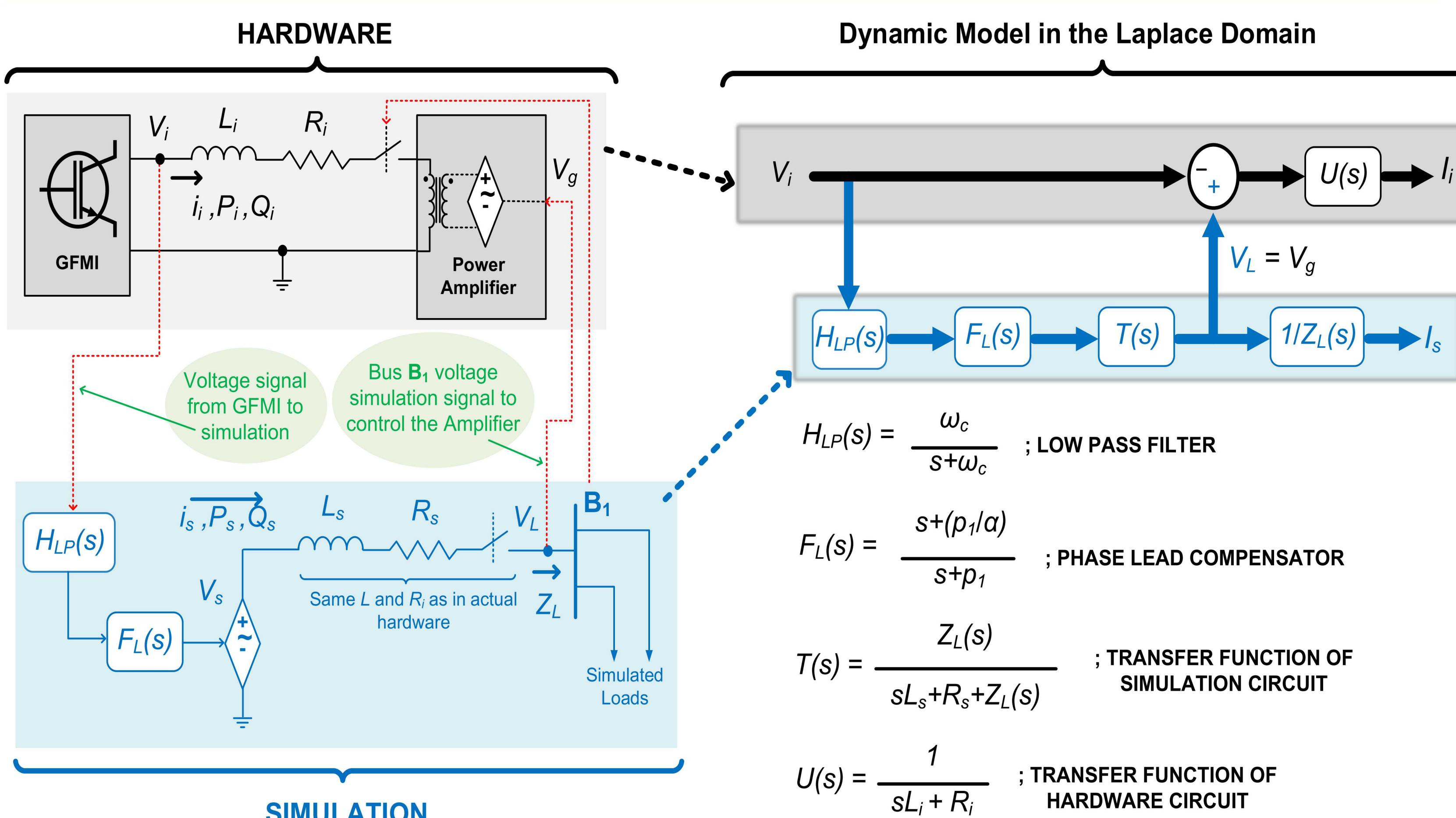
An external inductor ( $L_i$ ) is placed between the GFMI and the power amplifier. The voltage at the terminals of the GFMI is sensed and injected into simulation model, this marks a fundamental difference with the ITM. A digital twin of the hardware circuit is created at simulation level. If  $L_i=L_s$ ,  $R_i=R_s$ , and if  $V_L$  drives the power amplifier, then the power amplifier acts as a voltage-programmable load whose P and Q are equivalent to simulated loads at B1.
