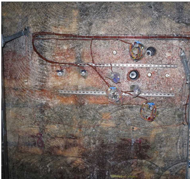
Heated BATS array, photo by Brian Dozier (WIPP TCO)
