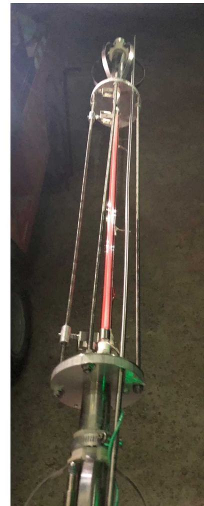
Infrared heater in BATS HP borehole
