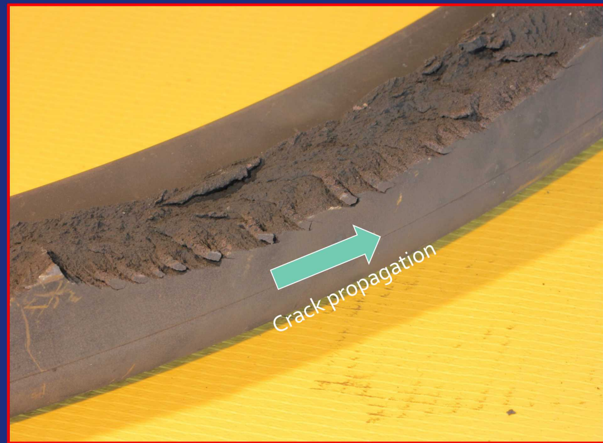
Figure 3. Detail of section showing clear direction of crack propagation (red box in Figure 2.)
