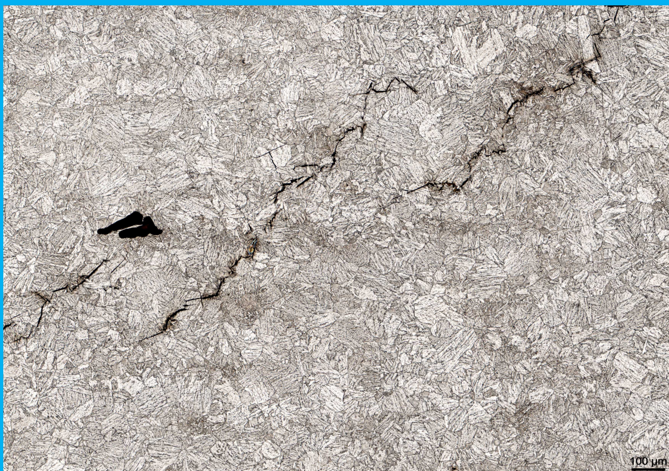
Figure 7. Microstructure is SOMETHING, secondary transgranular cracks are visible .
