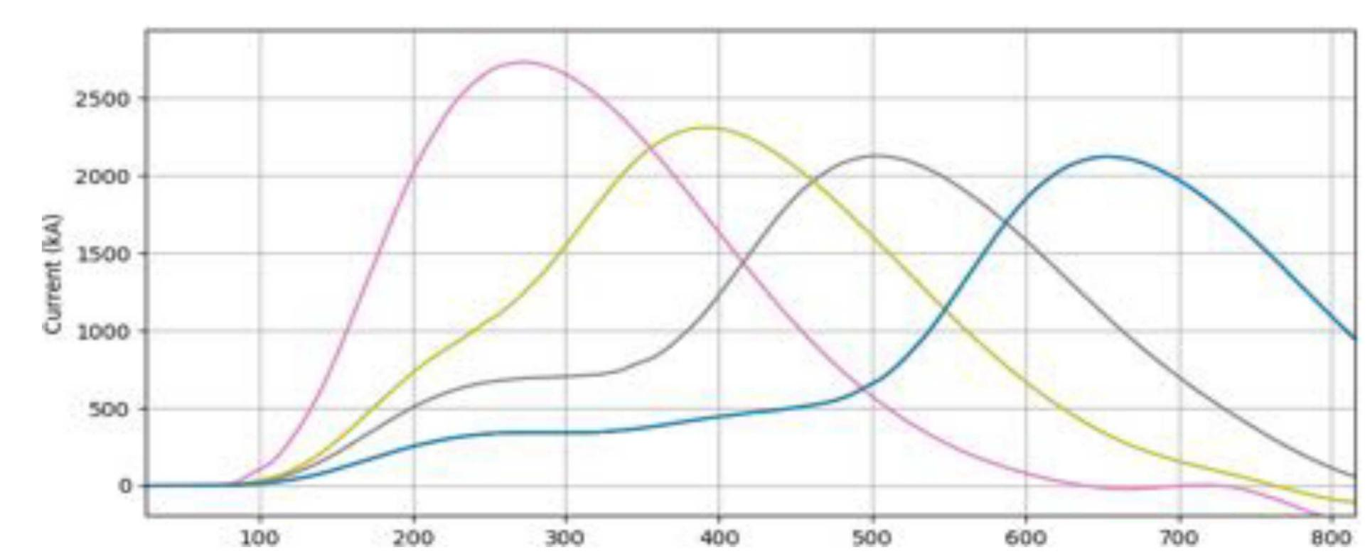
Fig. 13: A range of different pulse shapes. When all bricks are fired at once, the pink curve is produced (maximum current for Thor-64). When they are fired sequentially the timing and amplitude of the pulse shape can vary.
