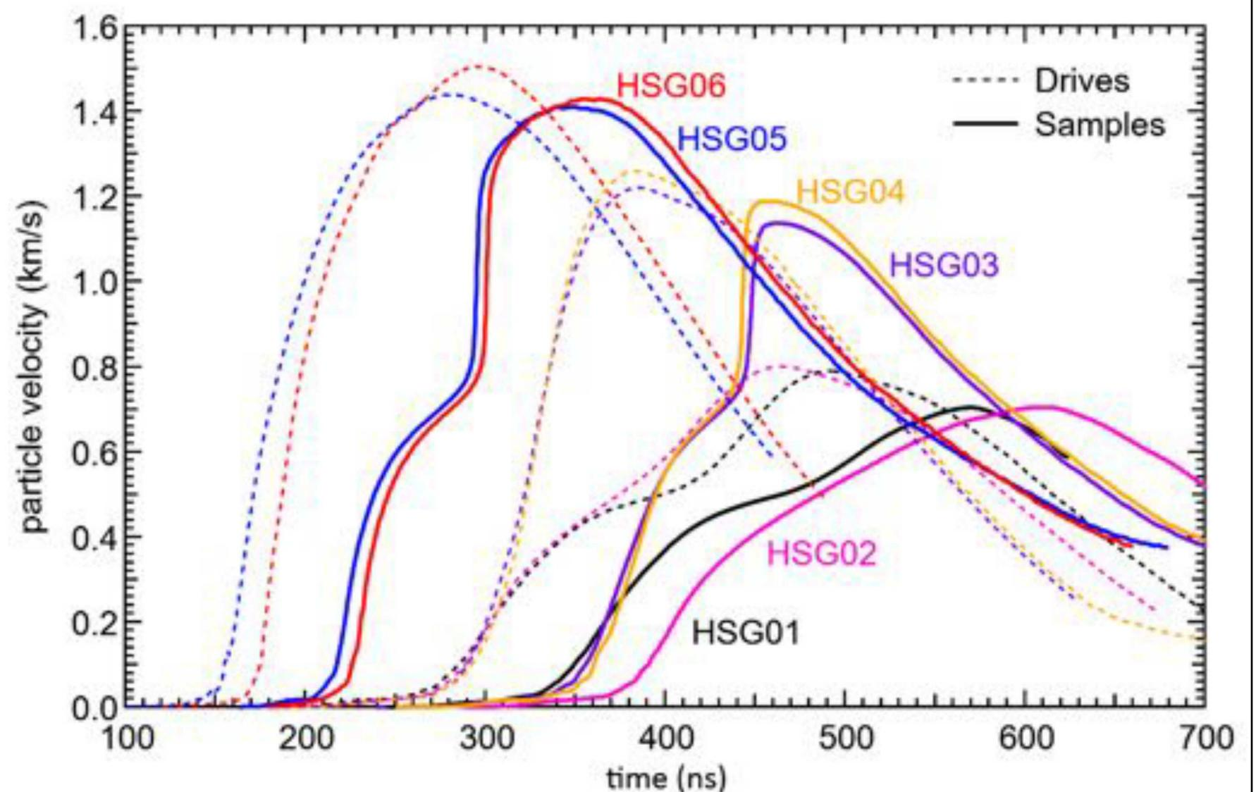
Fig. 15: Pulse shape for the drive (dashed) and sample response for six completed shots on Thor.
