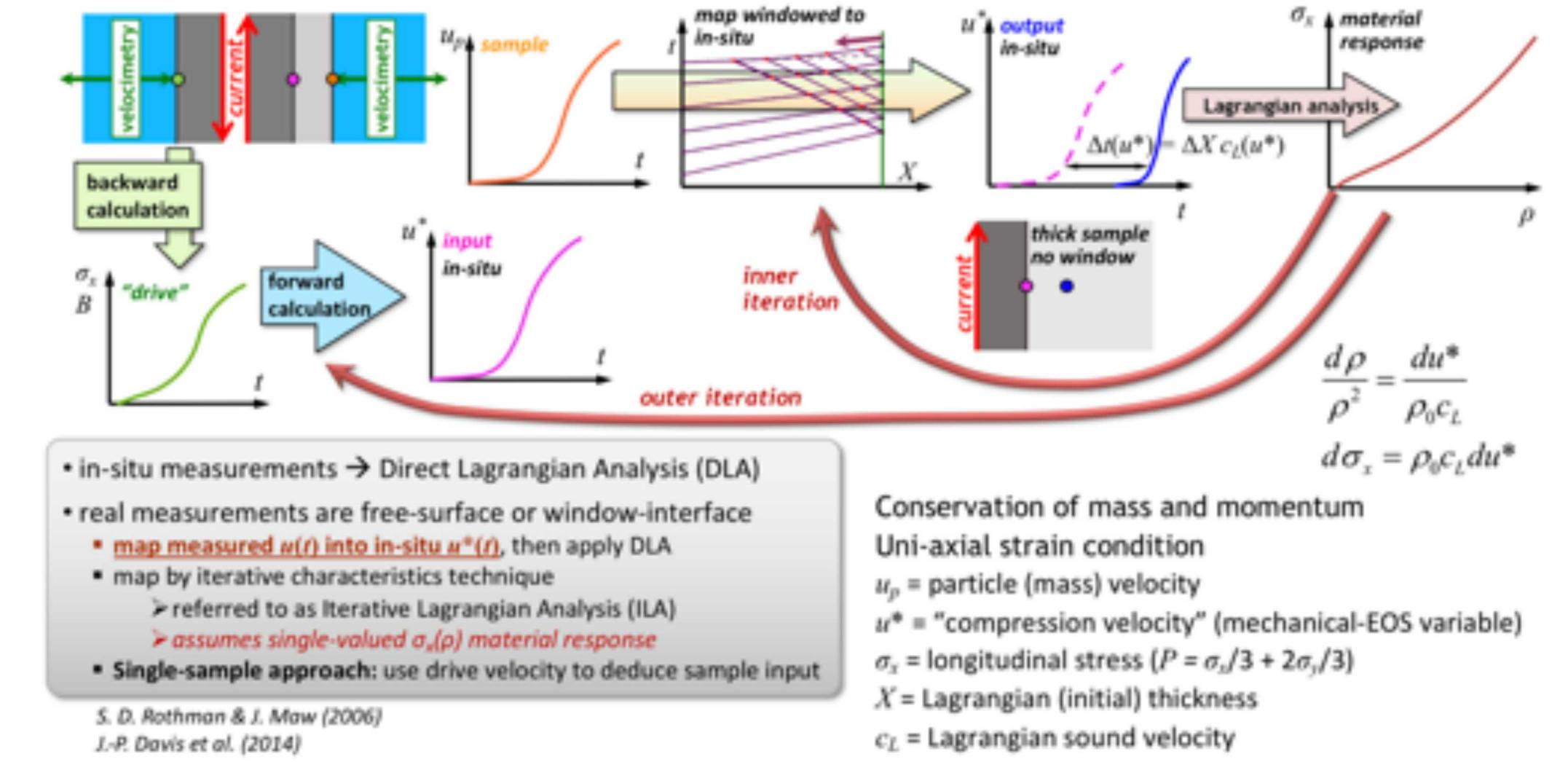
Fig. 14: Iterative Lagrangian analysis (ILA) determines stress-density path from velocimetry of LiF-windowed "drive" and sample. S. D. Rothman & J. Maw (2006); J.-P. Davis et al. (2014)
