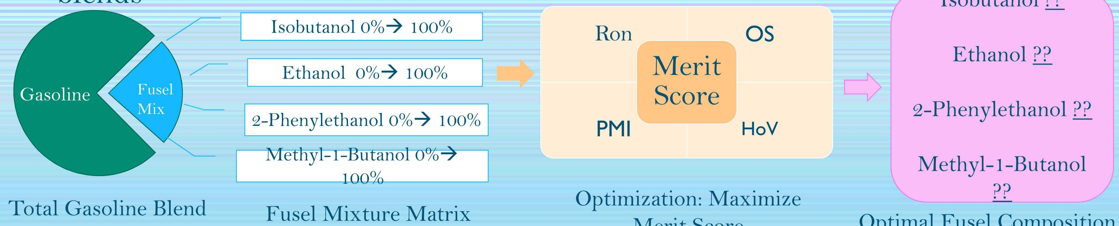
Flow chart depicting future workflow, beginning with the generation of a matrix containing the possible compositions of alcohol blends. The computational calculation of mixture properties will respectively generate a merit score for the wide range of mixtures to ultimately identify an optimal mixture or pareto front.
