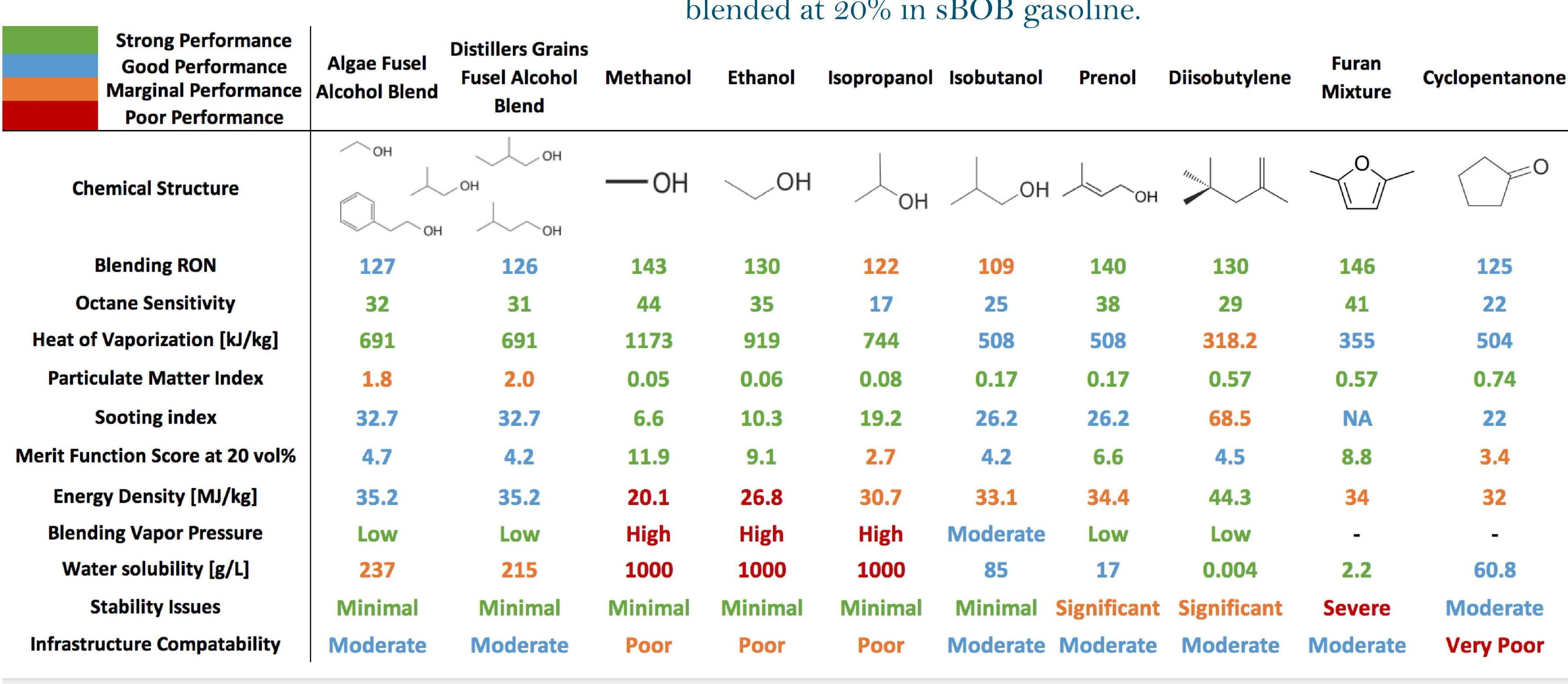
The above figure demonstrates the viability of fusel alcohol blends 4&5 as a gasoline blendstock in comparison to other top 10 blendstocks. Fusel mixtures 4&5 generally do not illustrate properties that contribute to poor performance, while other blendstocks have at least one poor performing property.
