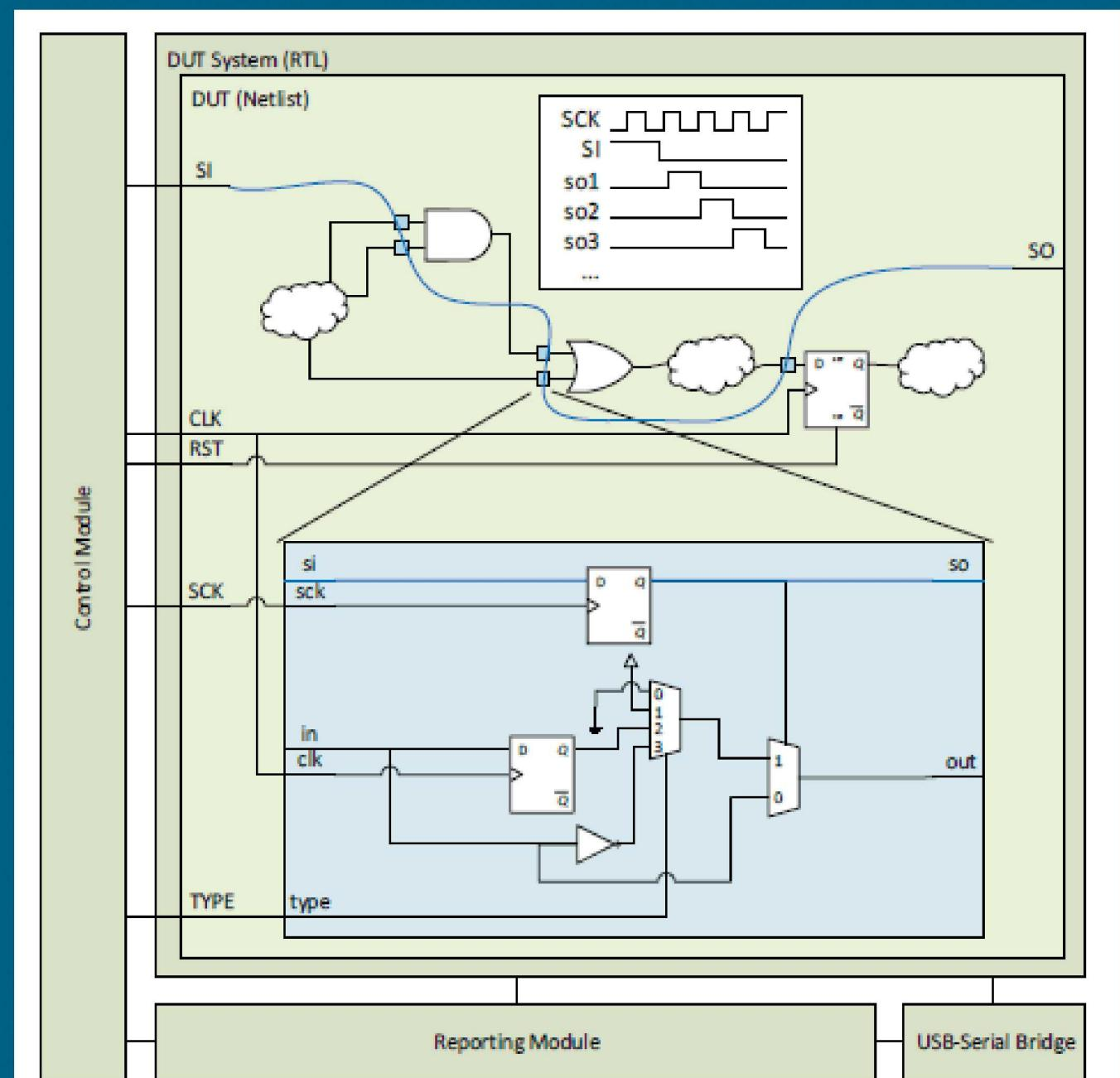
Device under test with saboteur circuits (blue) added to gate inputs.
