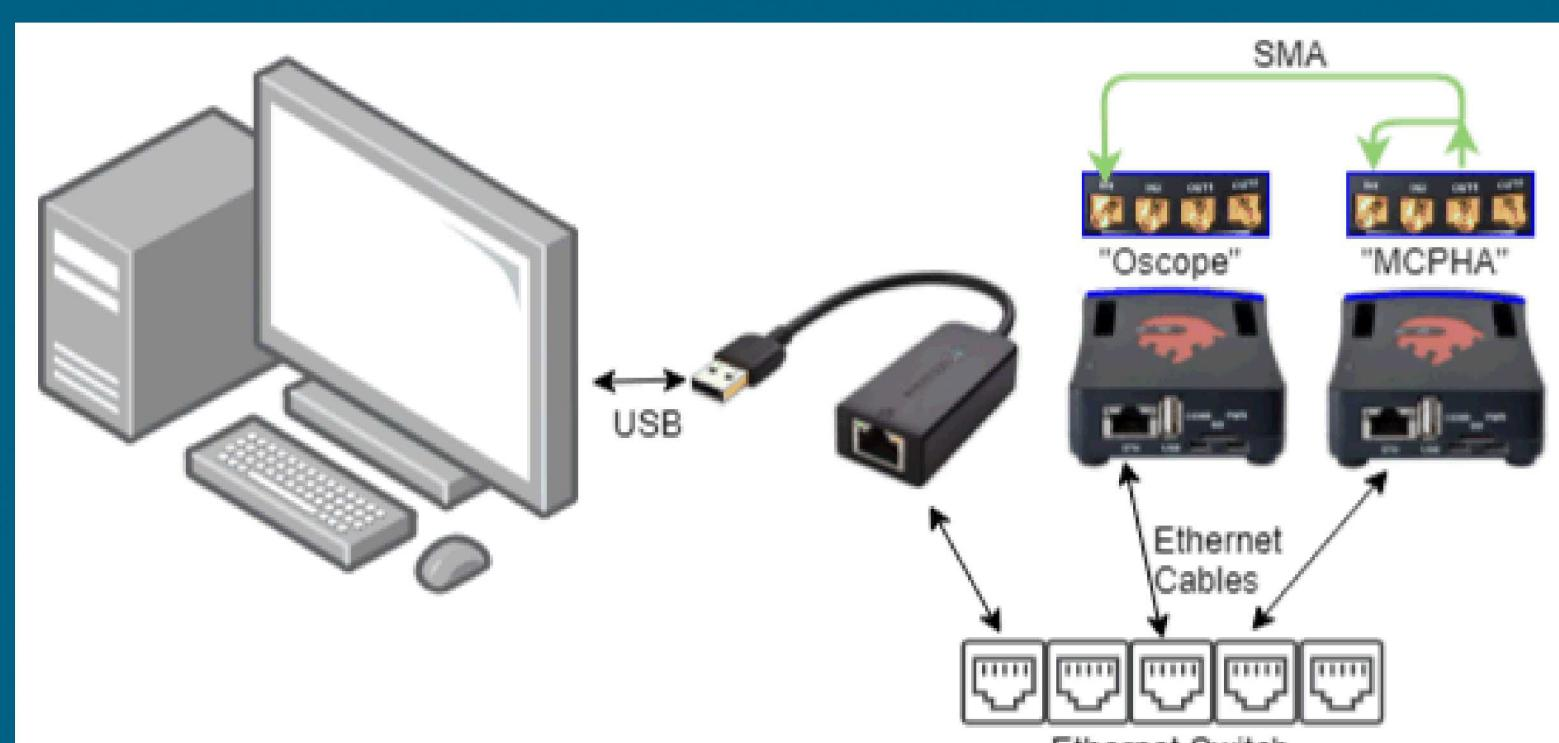
The signal generator Pitaya runs the server, which receives commands from the local machine running a python script/GUI.
