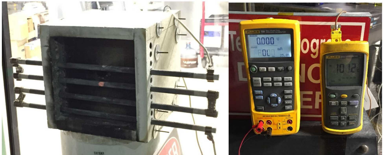
Fig. 5 Picture of the box heater used for the demonstration experiments (left) and its power control (right).
