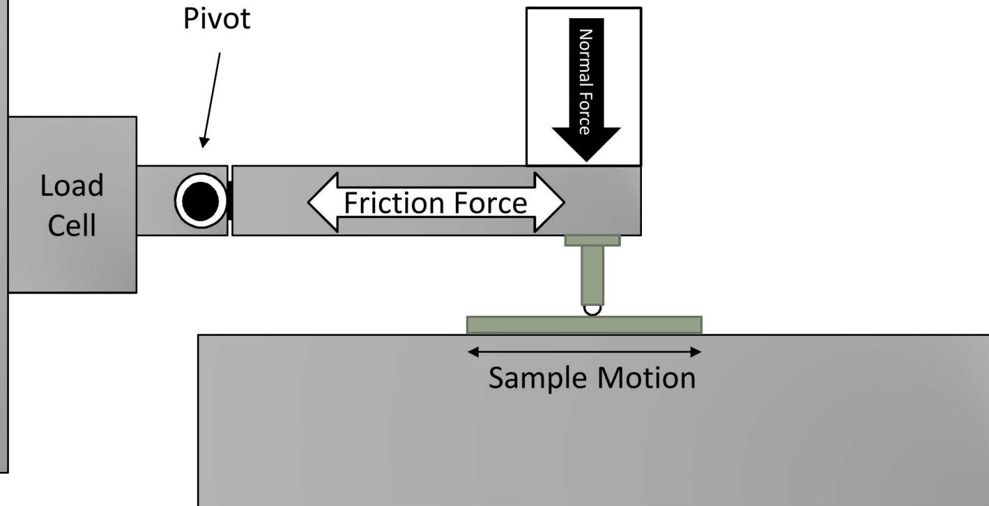
When sample moves underneath ball holder, friction force is resolved in rigidly mounted load cell. Bearing joint reduces the effects of misalignment and sample tilt.
