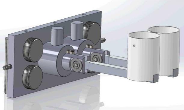
The tester is made of simple, dual load cell assemblies. Which are adjustable to accommodate different sample geometries and sizes.
