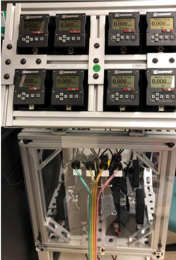
Each set of two flow meters (dry and humid) mixes to form one gas stream for each module (with a prescribed humidity). User can vary humidity by changing respective flow rates of dry and humid gas. Humid gas is created by flowing dry gas through bubblers which must be manually refilled.
