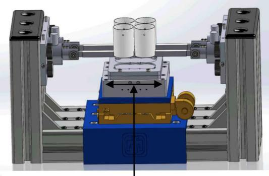
A single linear motion stage is paired with two load cell modules to create a “parallel” friction tester with the ability to test four samples simultaneously.
