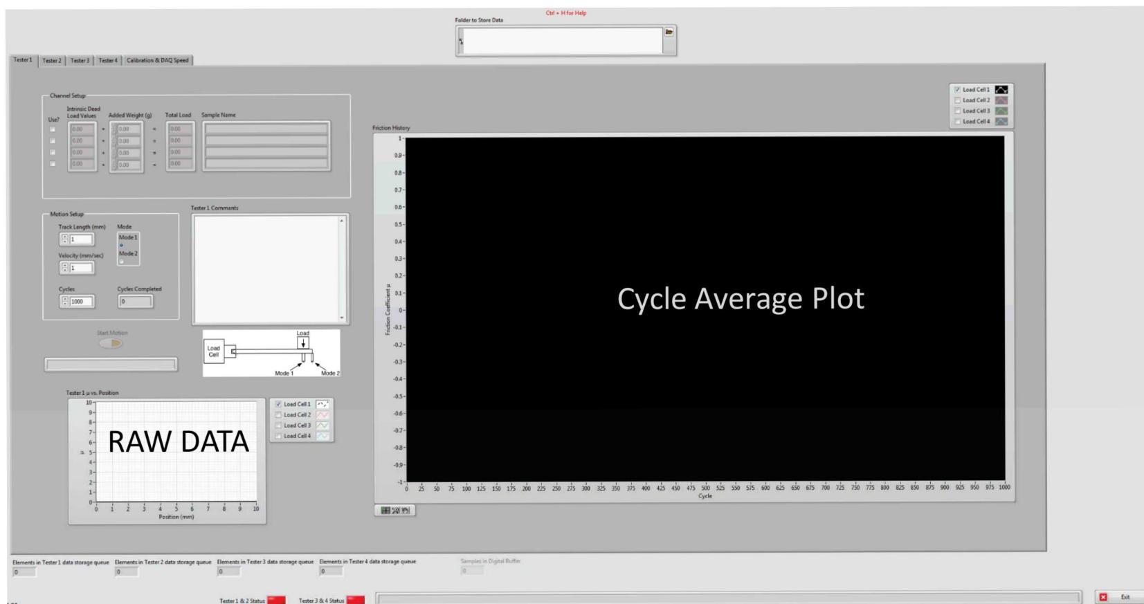
Software makes test monitoring easy. Plots last cycle's raw data to enable user to see whether tester is operating normally and as expected. User can be informed of “red flags” in raw data during training.
