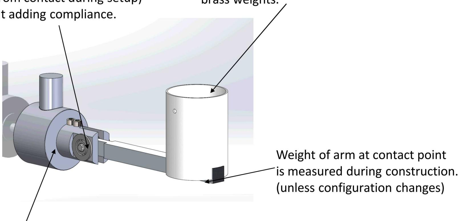
Load Cell is calibrated for tension/compression. When sample slides underneath contact, tension/compression is exerted on load cell.
