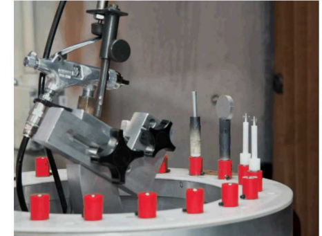
Spray \text{MoS}_2 + C with polymer binder
