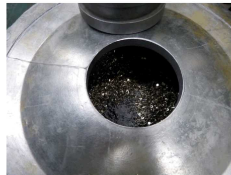
Parts tumbled in drum with \text{MoS}_2
