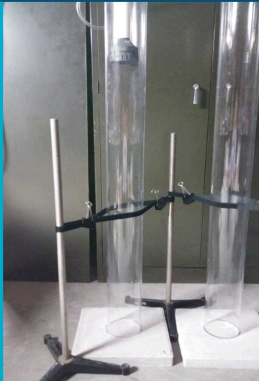
Resuspension chamber with vacuum pump head.
