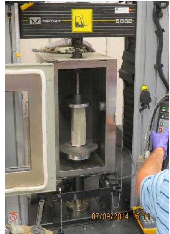
Compression Tests of Wind Turbine Blade Carrots
