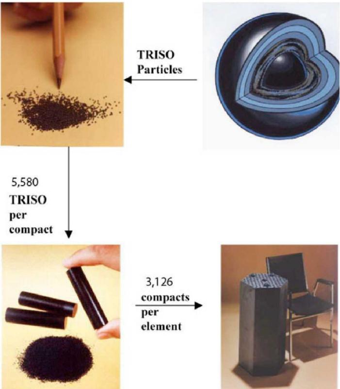
Characteristics of TRISO fuel with a  $UO_x$  core of radius 250 - 300  $\mu\text{m}$
