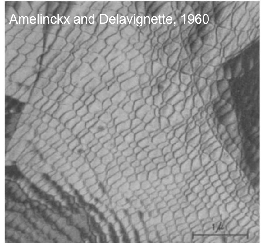
Fig. 1. Dislocation network in \text{Bi}_2\text{Te}_3 . Note that certain segments of dislocations and certain node-points have left the foil
