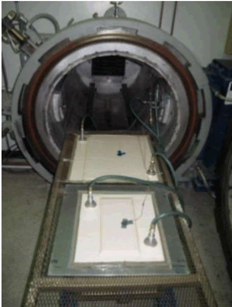
Panels Autoclave Cured
