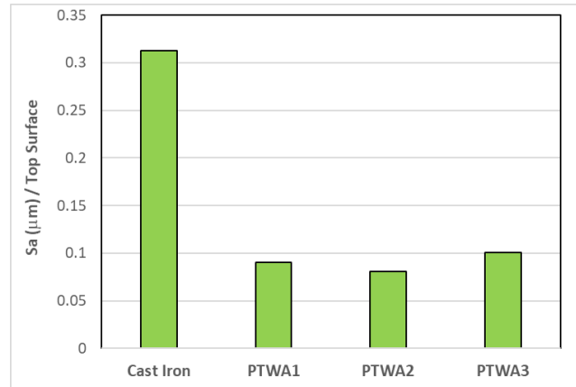
Figure 27. The surface finish of high porosity PTWA coatings excluding pores on the surface.
