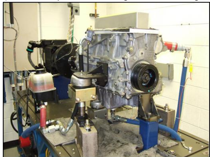
Figure 8. Motorized cranktrain assembly.
