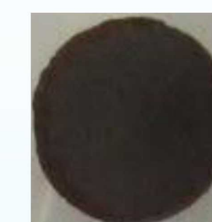
TCNQ@Cu-MOF-74 pellet ( d=1\text{cm} , b=0.0288\text{mm} )
