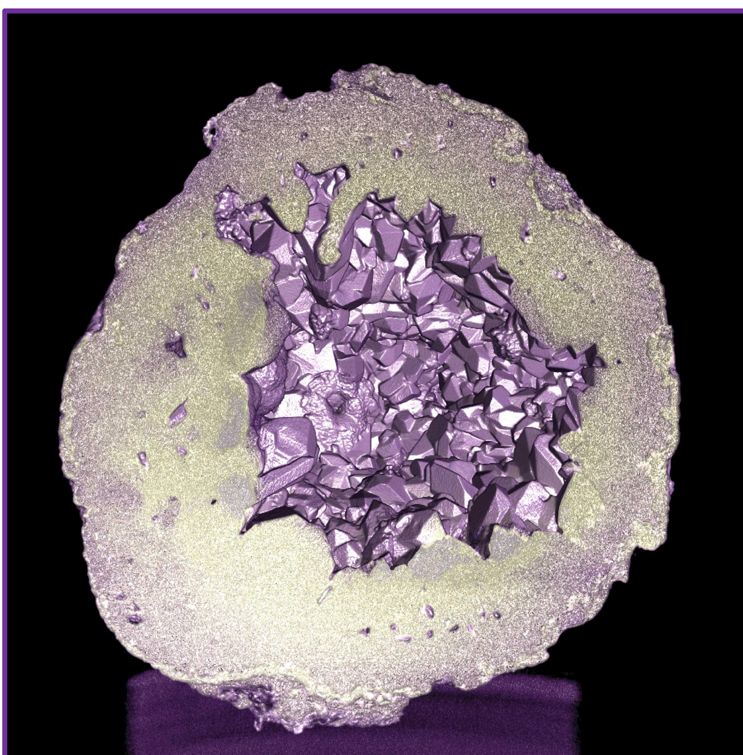
The Geode was shot using a 225 kV X-Ray Worx system with a Varian 2520DX detector
