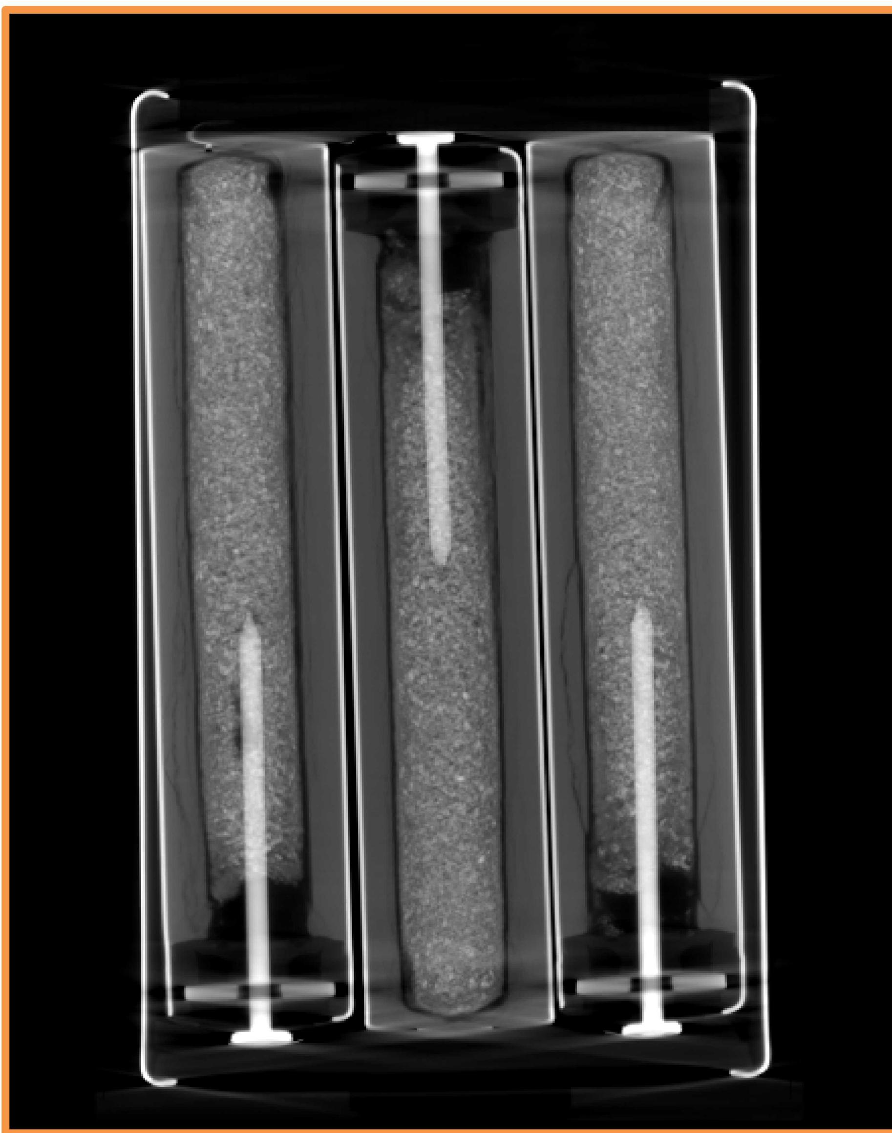
The battery was shot using a 225 kV X-Ray Worx system with a Varian 2520DX detector
