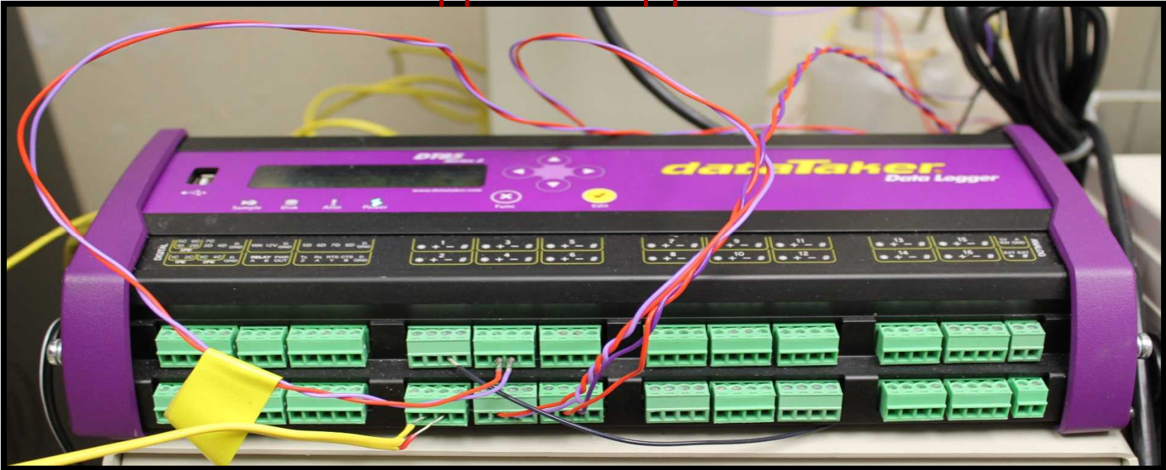
The Data Logger Unit
