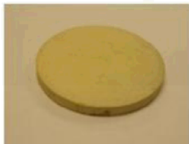
50 wt% AgI/50 wt% Glass, 500°C for 3 hr
