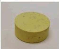
50 wt% AgI/50 wt% Glass, 500°C for 3 hr
