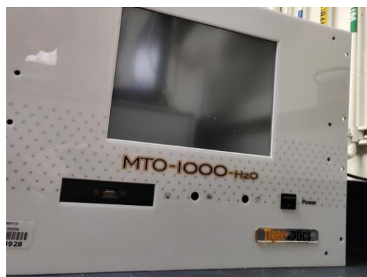
Figure 1-13. Tiger Optics MTO-1000-H 2 O setup for optically measuring PPM down to sub-PPB levels of water vapor in various (Ar, CO 2 , air) tank gases (before and after using water removing filters) that are being equilibrated with molten chloride salts.
