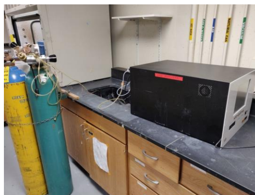
Figure 1-13. Tiger Optics MTO-1000-H 2 O setup for optically measuring PPM down to sub-PPB levels of water vapor in various (Ar, CO 2 , air) tank gases (before and after using water removing filters) that are being equilibrated with molten chloride salts.
