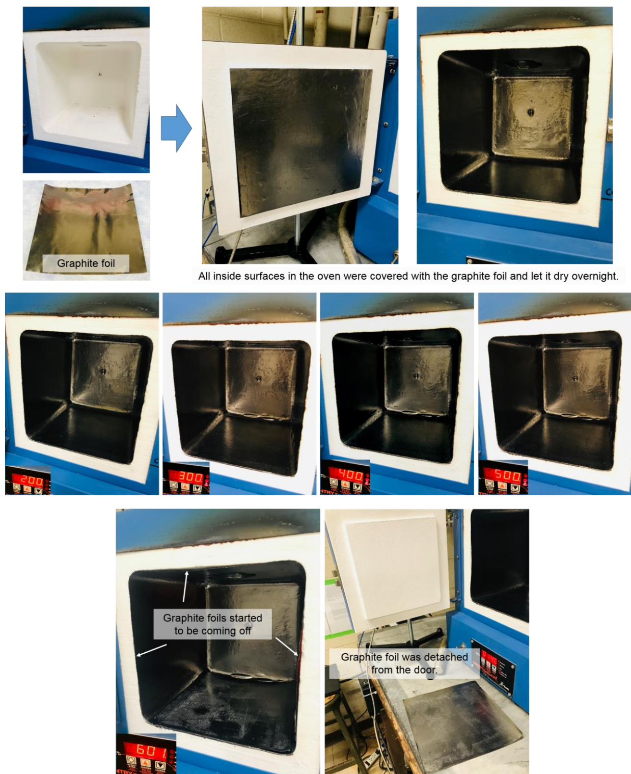
Figure 1.25 All inside surface in the oven covered with graphite foils. The graphite foils are stable from 25 to 600°C, so the Raman experiment can be run up to 600°C by covering the oven surface with graphite.
