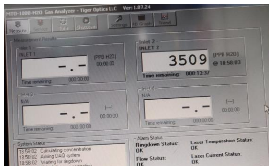
Fig. 1-14. TigerOptics detected 3.5ppm of water vapor in Argon tank gas.
