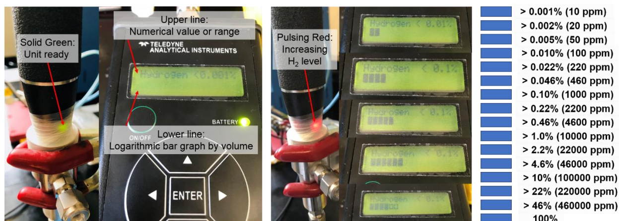
Figure 2-5. Pictures of the hydrogen sensor showing how the instrument detects and reports the hydrogen concentration near the probe tip.
