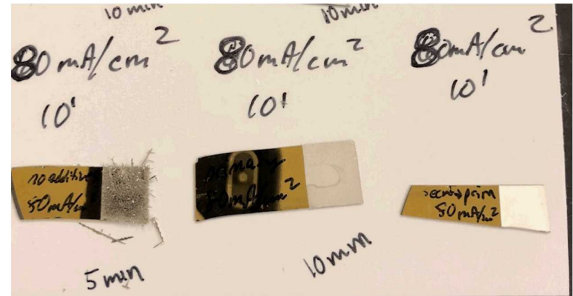
Electroplated tin with 80 mA/cm 2 current
