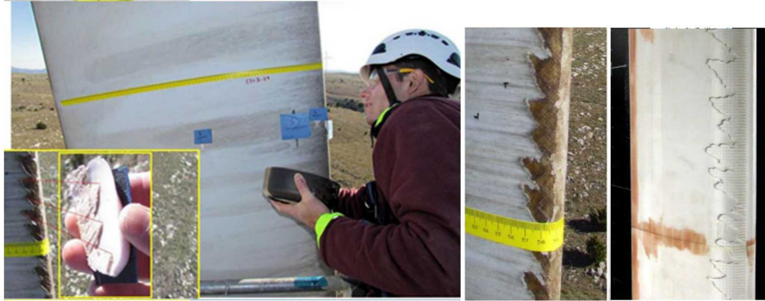
Figure 1. Category 4 damage from which an imprint reproduction of the eroded leading edge was tested in the wind tunnel [9, 12].
