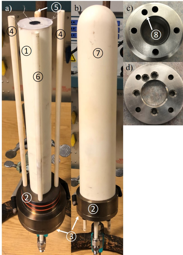
Figure 3. Button cell in the test fixture: a). Set up for testing in air. b). For testing in controlled atmosphere, an alumina tube with one closed end was placed over the set-up shown in a). c) Top view, upper part of the fixture. d) Top view, bottom part of the fixture. ① YSZ tube with cell sealed on top; ② Upper part of the test fixture; ③ Bottom part of the test fixture; ④ Double bores tube for electrode leads; ⑤ Type R thermocouple; ⑥ Cathode gas inlet tube; ⑦ Closed-end tube; ⑧ Cathode gas exhaust hole.
