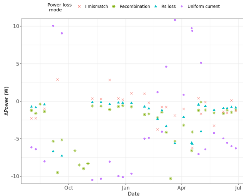
Figure 2: Power loss mechanisms from outdoor Suns-V_{OC} analysis.
