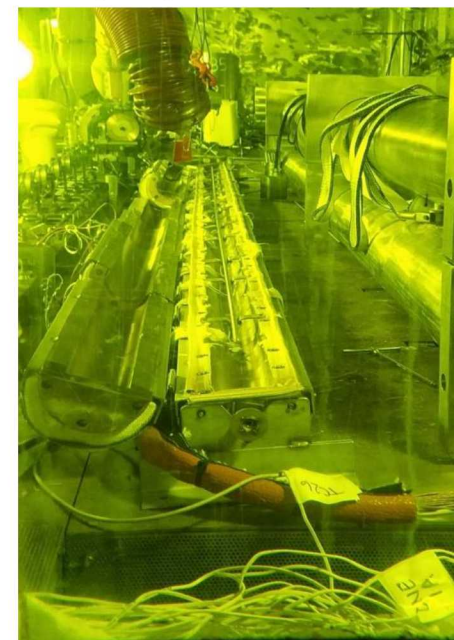
"Flattened" waterside surface of one of the sibling rods (above) and the ORNL full length rod heat treatment oven (below). Photos from Rose Montgomery, ORNL.
