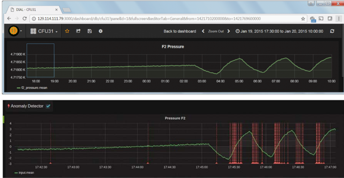
Figure 7. Use of z -score algorithm to detect point anomalies. Top panel: raw pressure data stream from one of the monitoring wells during pulse experiments, in which the injection rate was modulated to create pressure anomalies (i.e., the sinusoidal waves shown in the later times). The entire data length is about 16 hours and the first 90 min of data were used to train the algorithm; Bottom panel: detected anomaly (dashed pink vertical lines).
