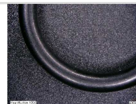
BR018-C failed at 132 cycles, -40°C
