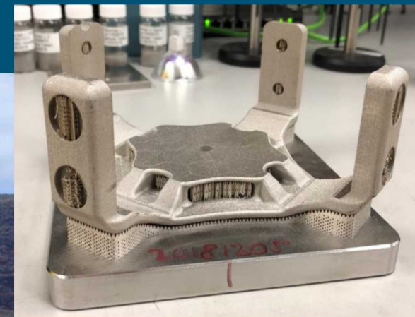
316L SS HOT SHOT top cap on plate
