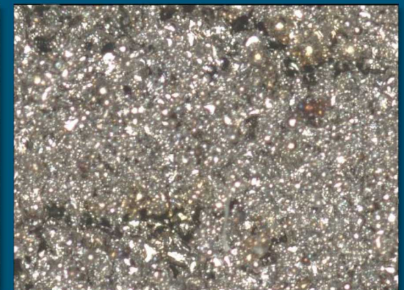
60.1W, 300mm/sec 891 \mu m PV form (left), top 73.8 \mu m Sa roughness (center), side 38.1 \mu m Sa roughness (right)
