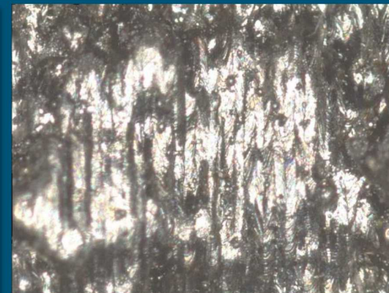
60.1W, 300mm/sec 891 \mu m PV form (left), top 73.8 \mu m Sa roughness (center), side 38.1 \mu m Sa roughness (right)
