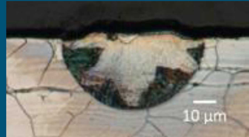
melt pool on plate, 100W, 1500 mm/s
