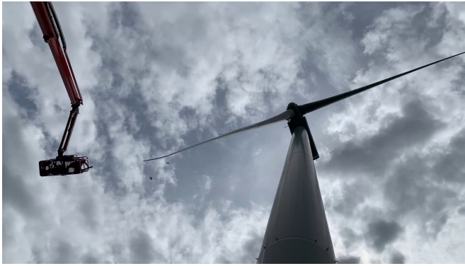
Fig. 4. Surrogate projectiles, such as tennis balls, were launched into the swept blade path of the operating wind turbine in order to simulate an avian collision with the turbine blades. Projectiles were launched from a compressed air cannon located on a nearby vertical personnel lift.
