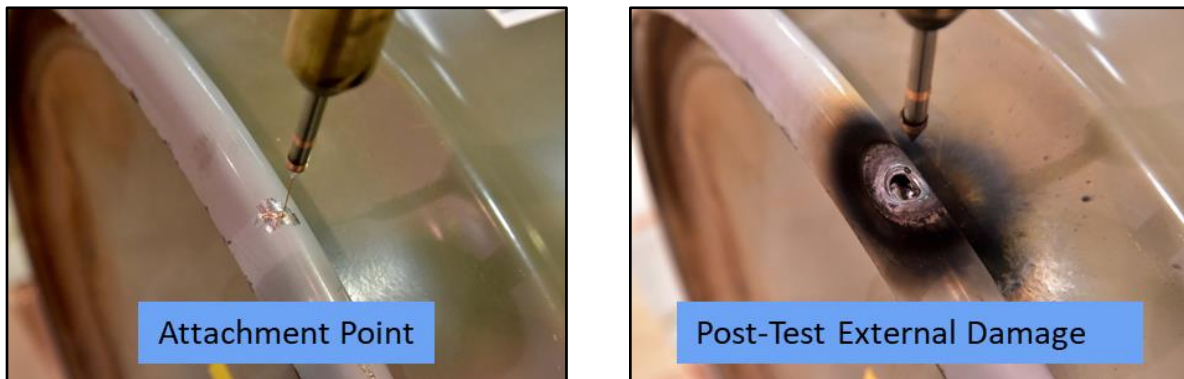
Figure 3-35. Attachment to TRU waste drum closure ring.
