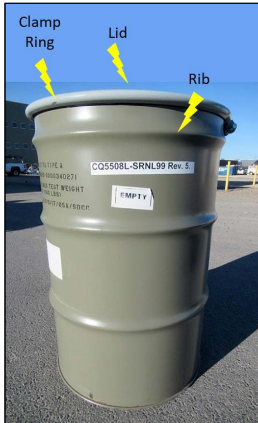
Figure 3-31. Lightning attachment points for 55-gallon drums.
