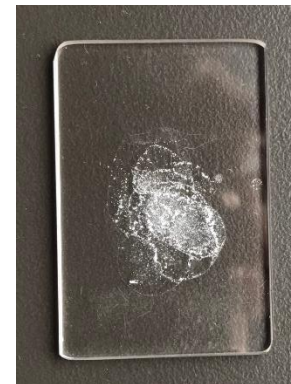
HREE+Y oxalate precipitates (~12%wt REY)
