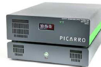
Picarro cavity ringdown Spectrometer (CRDS)
