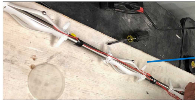
AE sensors on de-centralizers
