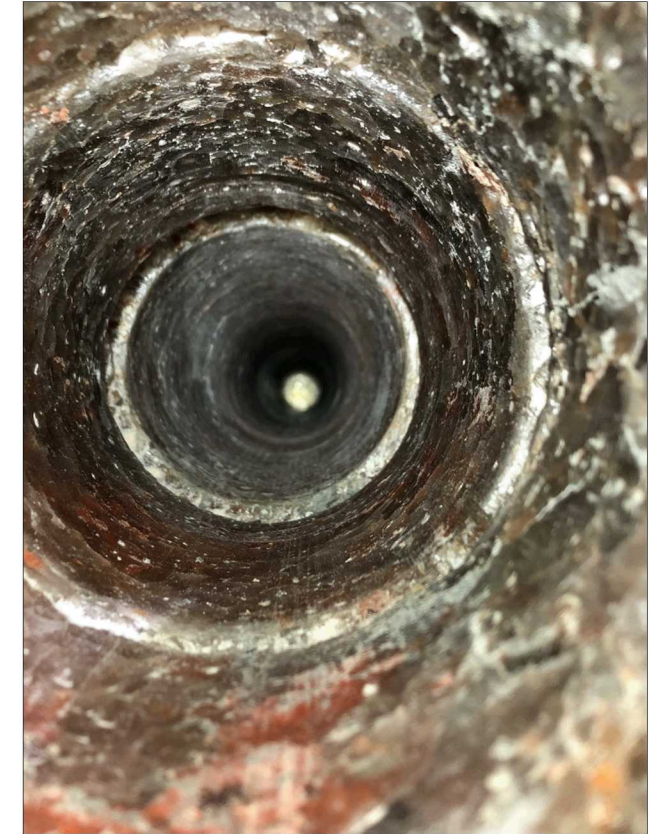
Discrete fractures in BATS near-drift EDZ
