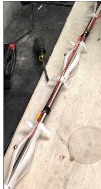
Decentralizers and piezoelectric transducers
