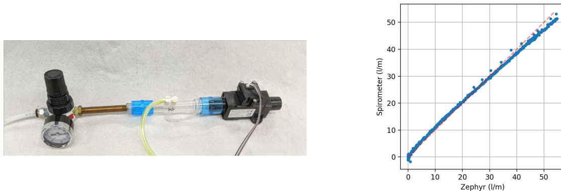
Figure 5: Calibration of the spirometer. (Left) calibration setup showing the spirometer in series with the Honeywell flow meter and a small pressure regulator to sweep the flow. The results are shown in (Right).
