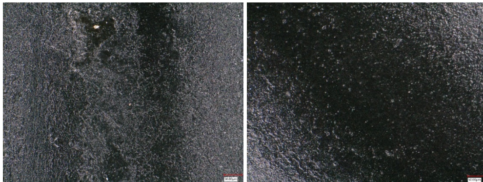
Figure 22. Optical microscopy pictures comparing Buna N from FN-C fueling nozzles (FN004 vs FN018) that were tested at 500 cycles (left) and 1000 cycles (right) at -20°C
