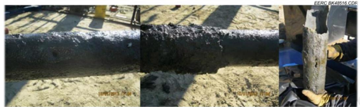
Corroded production casing pipe sample from downhole*
