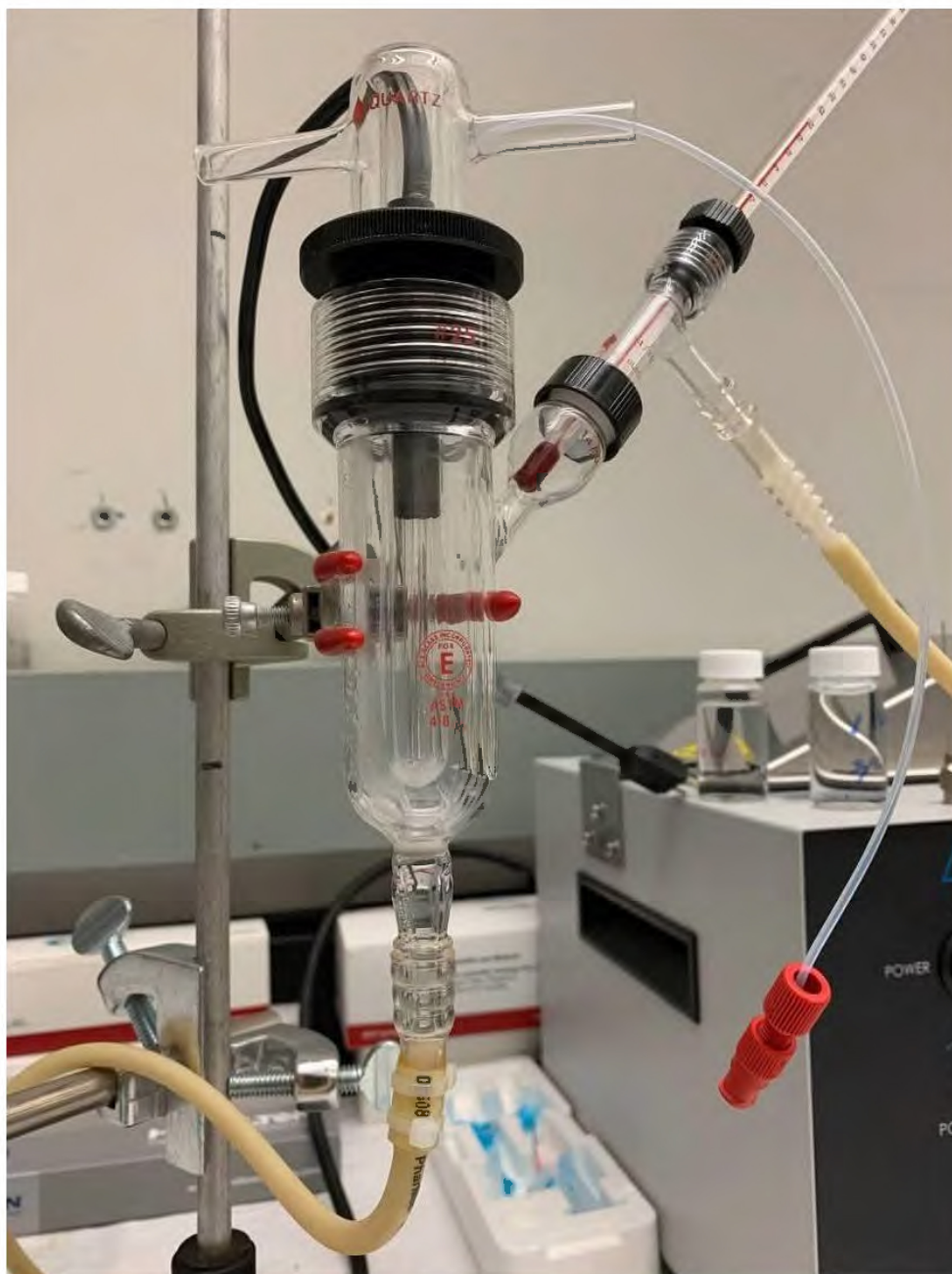
Figure 2.2. Micro-reactor assembly showing cooling jacket and syringe sampling line.
