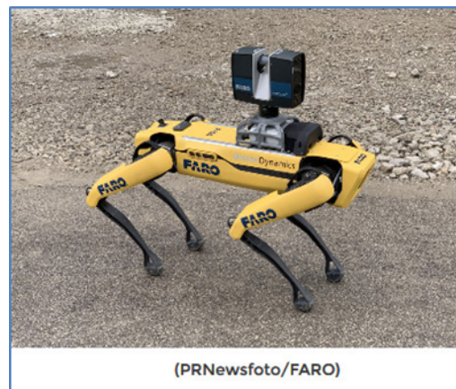
Figure 30. FARO Trek; a LiDAR scanner on a mobile platform
